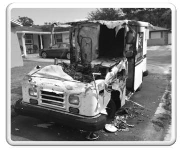
The Long Life Vehicles are way past their life expectancy. With worn parts, corroded wires, eroding insulation, worn out engines, and the summer heat, our LLVs are regularly overheating. This LLV fire, from Hilldale Station, is a result of overheating. The LLV got so hot the electrical wires caught fire. Fortunately no one was injured in this fire; the mail damage is secondary to the safety of the carrier.
